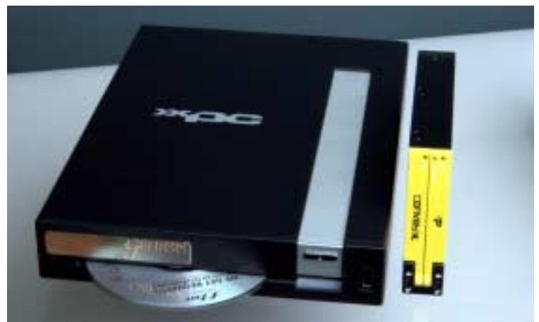
The Genesis Music Server is built around a Shuttle XPC and a 1 TB RAID D2 drive
