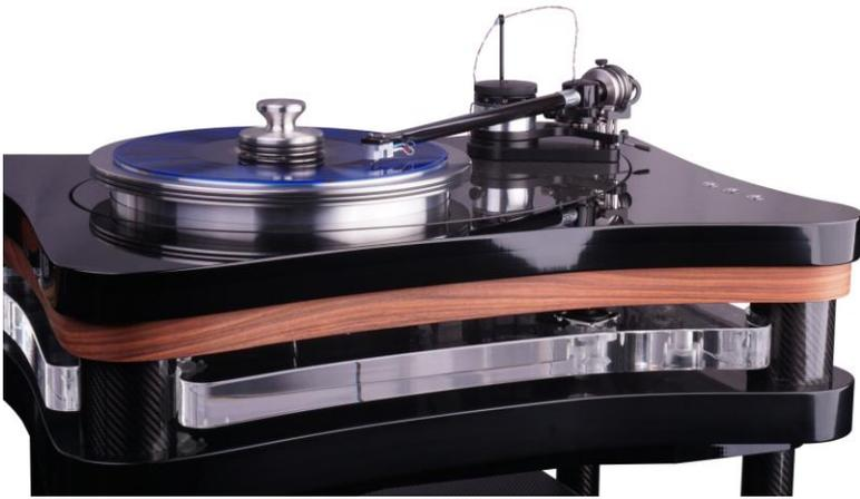
The main component of this vibration control is done using an 11-layer carbon-fiber composite and wood sandwich that we've developed over the past 10 years and used effectively for our loudspeaker cabinets. This is the plinth for the all-important motor/tonearm interface. The plinth is then spiked to a HMWA platform and this platform is hung from the superstructure with a low-Q low-compliance suspension system.
